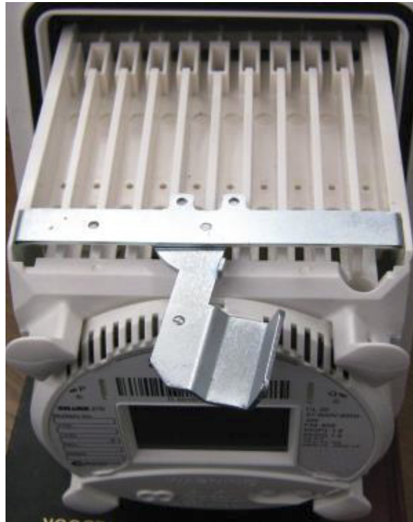
Figure 8.18: Removing the Cradle from the Switchboard Case
